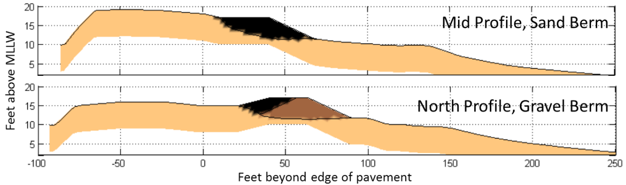
Figure 26: XBeach Model Substrate Variability with Design Alternatives
